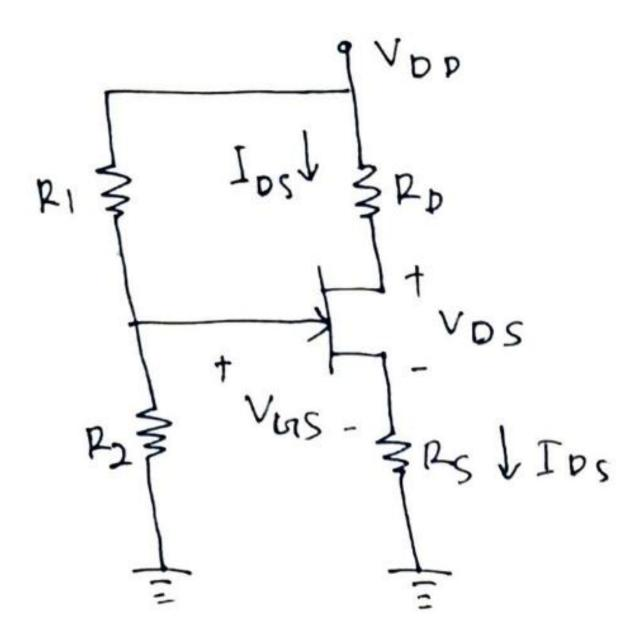
R, & R2 forem voltage divider Applying voltage division rule
