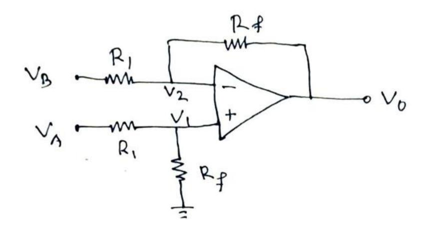
IZ R-1 voltage division rule at V, RI  $V_{1} = \frac{V_{A} + \mu_{f}}{R_{f} + R_{1}}$ V2 + Vol Rf V2=V1 (According to Virtual ground )
